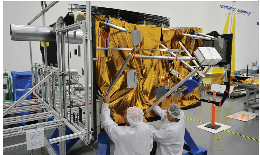
Technicians at Northrop Grumman Aerospace Systems facilities [above] in Redondo Beach, Calif., work on a mock-up of the JWST spacecraft bus—the home of the observatory's power, flight, data, and communications systems. The Earth-sun Lagrange points [below] are equilibrium locations where competing gravitational tugs on an object do not disturb its once-a-year orbit around the sun. JWST is one of three craft currently orbiting L2.
