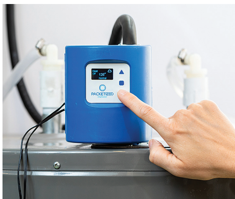
This controller connects to a residential electric water heater and uses simple algorithms to request “packets” of energy from a cloud-based coordinator to maintain a suitable temperature.
