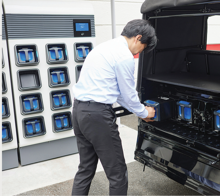
A Honda researcher inserts a charged Honda Mobile Power Pack battery into an e-rickshaw.
