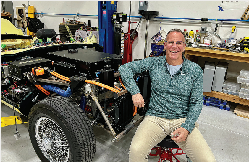
In his workshop, venture capitalist Adam Grosser is converting the original drivetrain on his 1974 Jaguar E-Type to an electric one.
