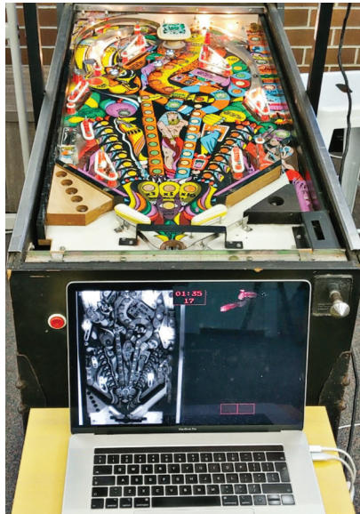
Pinball is a simple test of neuromorphic systems. It's so simple, in fact, that we built a two-artificial-neuron system that could keep three balls in play at once.
