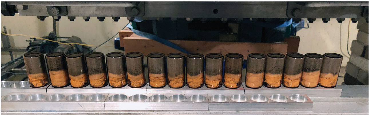
The deuterated erbium (chemical symbol \text{ErD}_3 ) is placed into thumb-size vials, as shown in this set of samples from a 20 June 2018 experiment. At left, the vials are arrayed pre-experiment, with wipes on top of the metal to keep the metal in position during the experiment. The metal has begun to crack and break apart, indicating it is fully saturated with deuterium. Below, the vials are placed upside down to align the metal with the gamma ray beam. Gamma rays have turned the clear glass amber.
