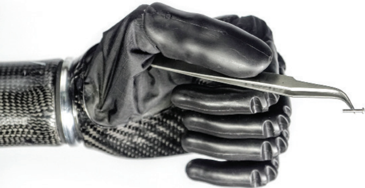
Psyonic's Ability Hand offers 32 different grips. It weighs around the same as an average adult hand.
