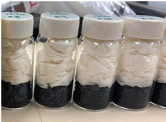
The deuterated erbium (chemical symbol \text{ErD}_3 ) is placed into thumb-size vials, as shown in this set of samples from a 20 June 2018 experiment. At left, the vials are arrayed pre-experiment, with wipes on top of the metal to keep the metal in position during the experiment. The metal has begun to crack and break apart, indicating it is fully saturated with deuterium. Below, the vials are placed upside down to align the metal with the gamma ray beam. Gamma rays have turned the clear glass amber.
