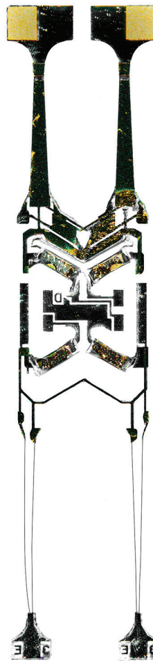
■ ■ ■ This quartz tuning fork responds to inertial forces and forms the heart of the GyroChip.
