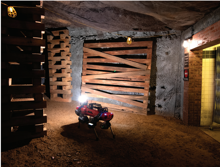
An ANYmal quadruped from Team Cerberus enters the course [top]. During the competition, only robots and DARPA staff were allowed to cross this threshold. The visual markers surrounding the course entrance provided a precise origin point from which the robots would base the maps they created. This allowed DARPA to measure the accuracy of the artifact locations that teams reported to score points. Cerberus's ANYmal exits the urban section of the course, modeled after a subway station [bottom], and enters the tunnel section of the course, based on an abandoned mine.
