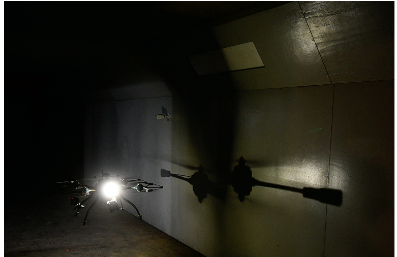
While most of the course was designed to look as much like real underground environments as possible, DARPA also included sections that posed very robot-specific challenges. Robots had the potential to get disoriented in this blank white hallway (part of the urban section of the course) if they couldn't identify unique features to differentiate one part of the hallway from another.
