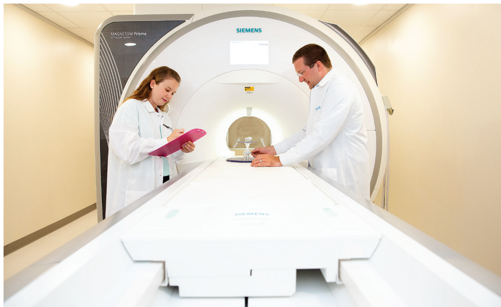
FIGURE 1 Engineers at MED Institute Inc. performing physical MRI testing to evaluate the safety of medical devices in the MRI environment.
