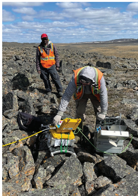
Audry Afango [far left] and Morgan McNeill work with a receiver on a ground electromagnetic loop in the middle of an angular boulder field in Nunavik, Que., Canada. On the right, McNeill, a geophysics technician, uses a superconducting quantum interference device (SQUID) to conduct a ground electromagnetic survey to pick up faint magnetic fields from conductive bodies underground.
