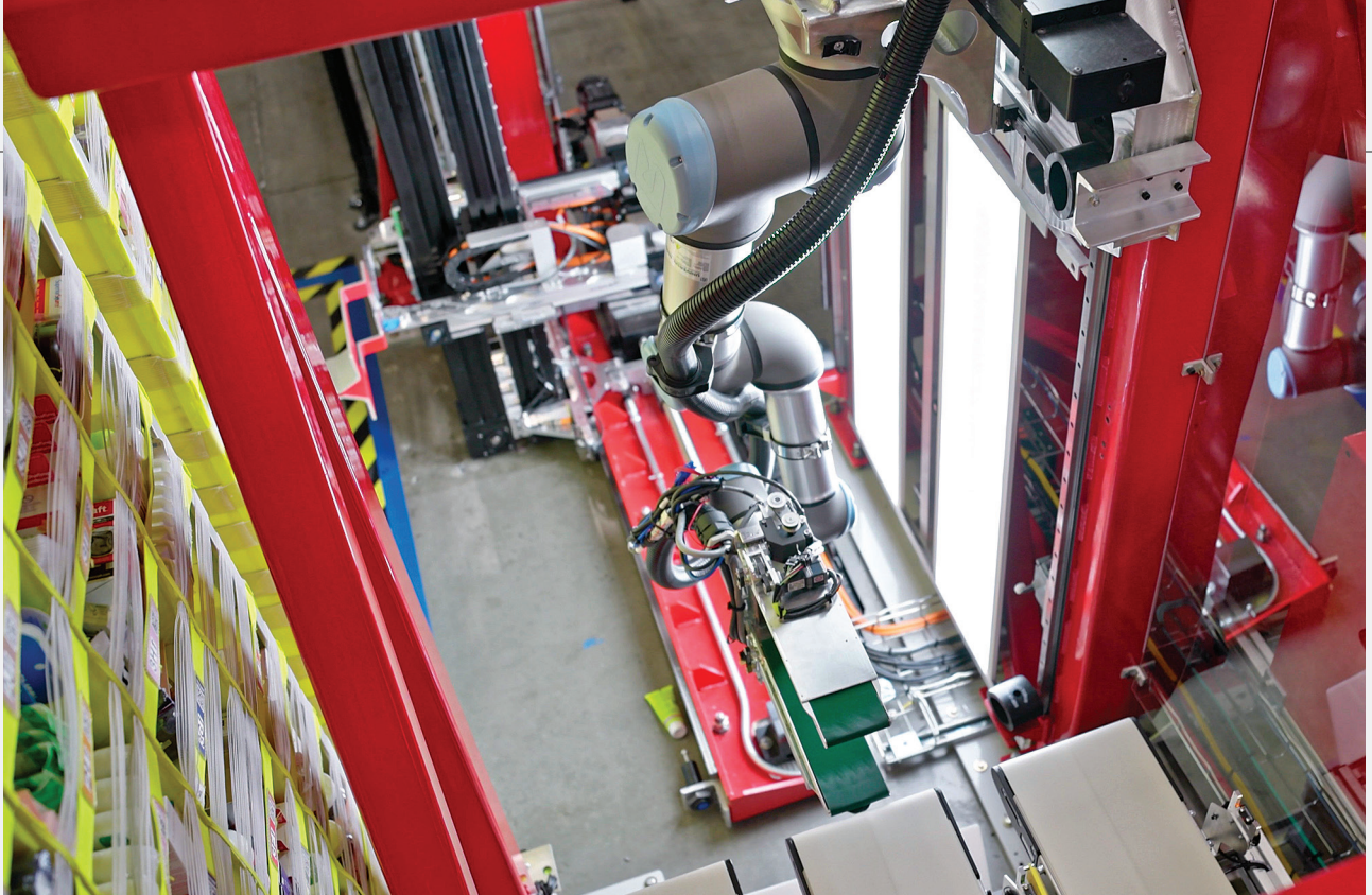
The robot includes a tool with twin conveyor belts [in green] designed to push items into storage bins.
