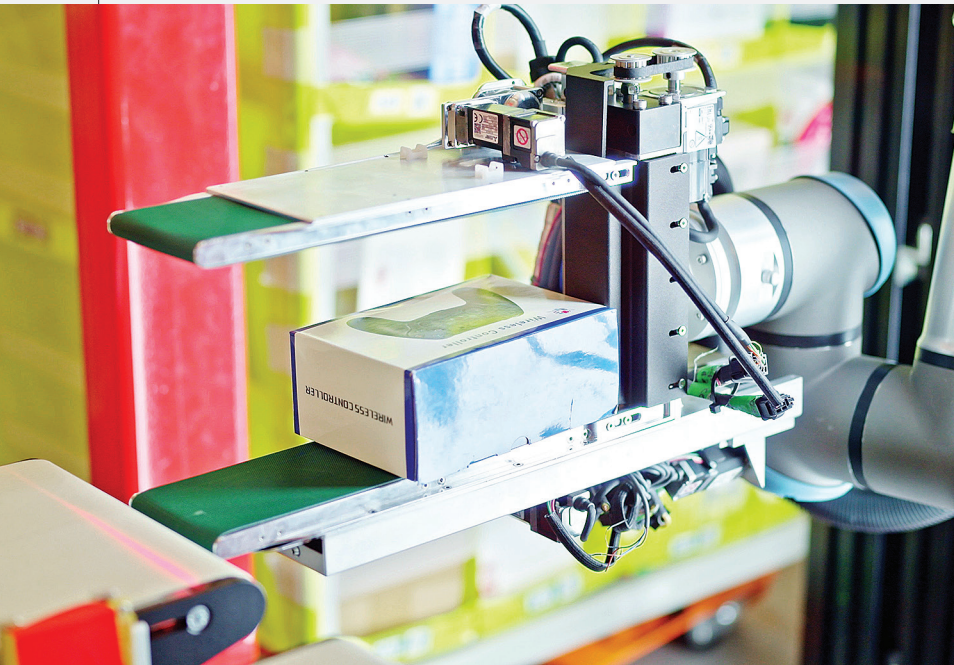
The end-of-arm tool (EOAT) is a key component of Amazon's new stowing robot.
