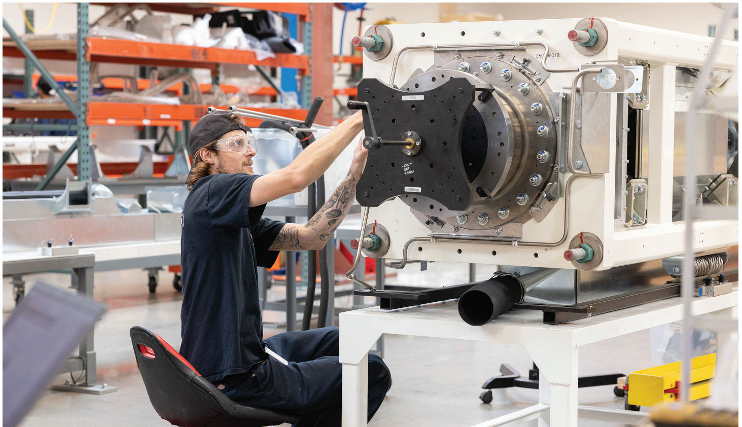
Linear generators are currently being manufactured at one of Mainspring Energy's facilities in Menlo Park, Calif. Clockwise from top left, technicians work on the frame of a linear generator core; a technician routes compressed air from an air spring to a generator's bearings; a gantry moves a completed core across the manufacturing floor for final assembly; another technician prepares copper wires to be wound into coils; and a stator is positioned in preparation for assembly. TOP ROW: CREATIVE SHOT; BOTTOM ROW: MAINSPRING
