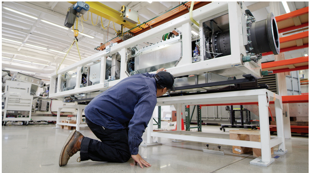
Linear generators are currently being manufactured at one of Mainspring Energy's facilities in Menlo Park, Calif. Clockwise from top left, technicians work on the frame of a linear generator core; a technician routes compressed air from an air spring to a generator's bearings; a gantry moves a completed core across the manufacturing floor for final assembly; another technician prepares copper wires to be wound into coils; and a stator is positioned in preparation for assembly. TOP ROW: CREATIVE SHOT; BOTTOM ROW: MAINSPRING
