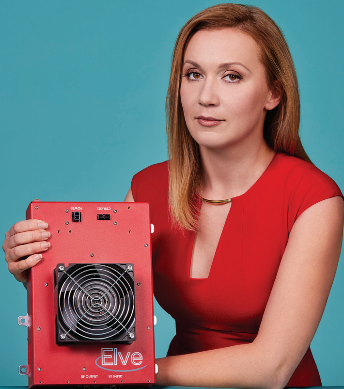
Founder Diana Gamzina holds Elve's millimeter-wave power amplifier system, which uses 100 watt E-band traveling-wave tubes.
