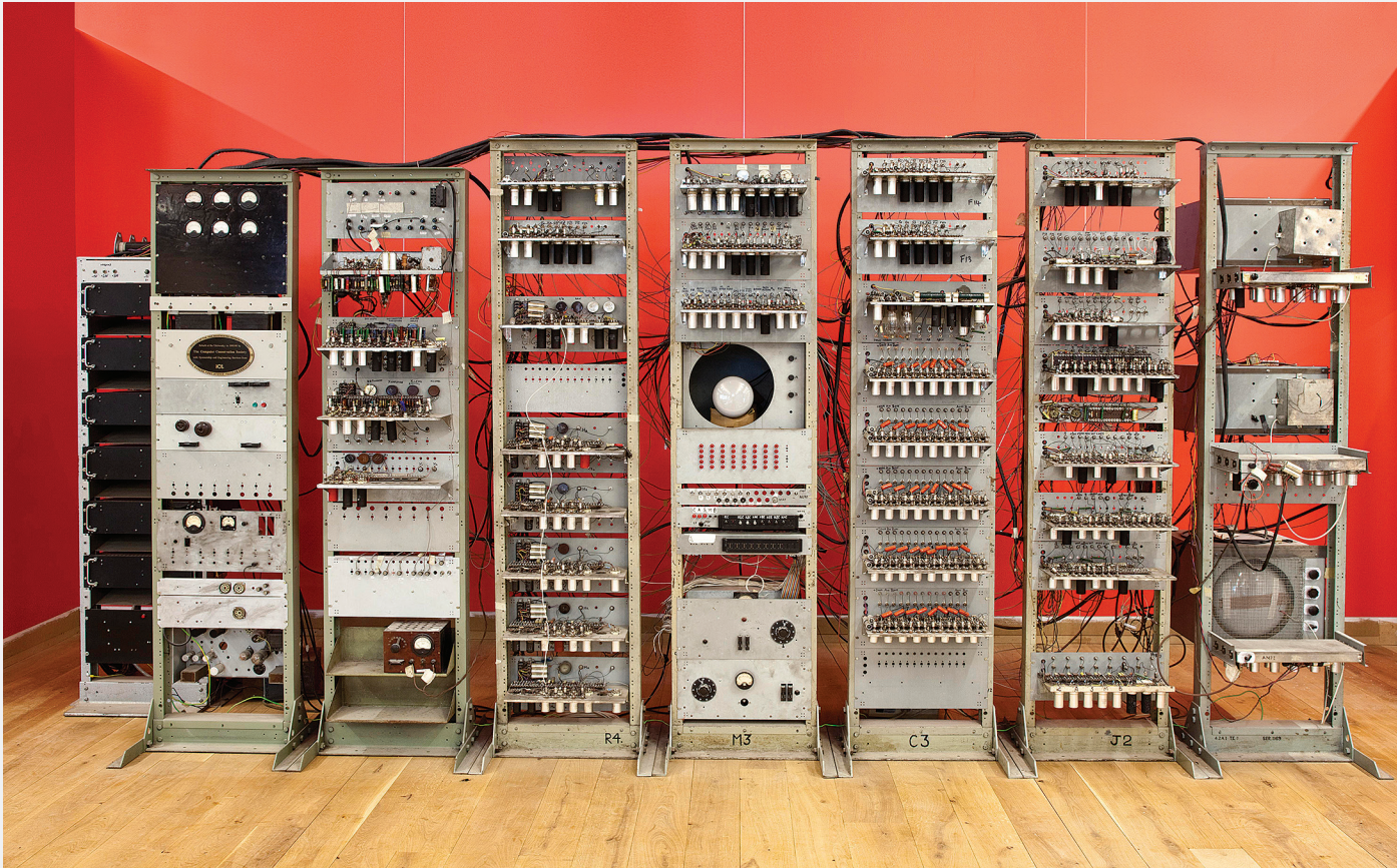
Weighing almost a tonne, the Manchester “Baby” computer was 5 meters long and 2 meters tall.
