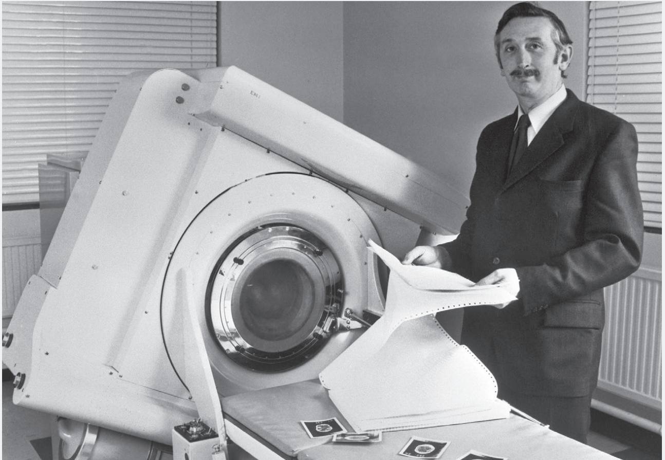
Research engineer Godfrey Hounsfield invented the CT scanner to create three-dimensional brain images.
