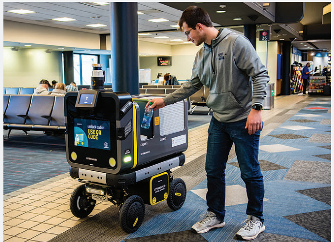
Ottobot can adjust its position and height so that anyone—including children, the elderly, and people with disabilities—can reach its cargo.
