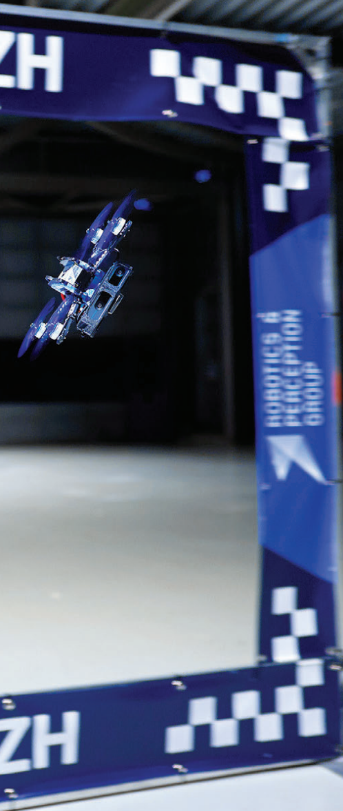
A human-piloted red racing drone chases an autonomous vision-based blue drone [left] through a gate at over 13 meters per second.
